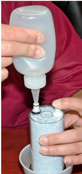
Figure 27 Checking desiccant for leaks
